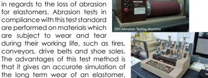
control of the uniformity of a specific material, and provides important parameters with respect to the wear of elastomers in practical use. The abrasion tester can also be used for comparative measurements on other materials such as plastics, chalk or painted surfaces.
