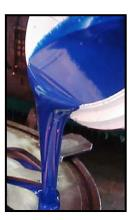
"Stripping" as it is known, is the physical process of reducing free TDI. It involves heating prepolymers up to temperatures well above 130°C. Instead of "Stripping" technology we have used our own expertise in chemically modifying the prepolymers design, to lower the Free TDI level in these new grades.
